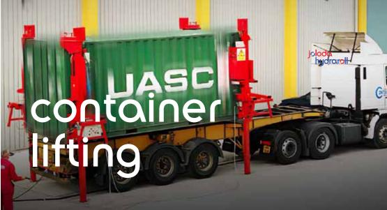
Similar in design to the Skate & Track system but with added hydraulics, this solution is specifically designed for loading sea and box containers.
