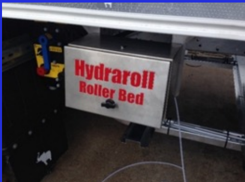
STAINLESS STEEL CONTROL BOX UNDERNEATH VEHICLE
