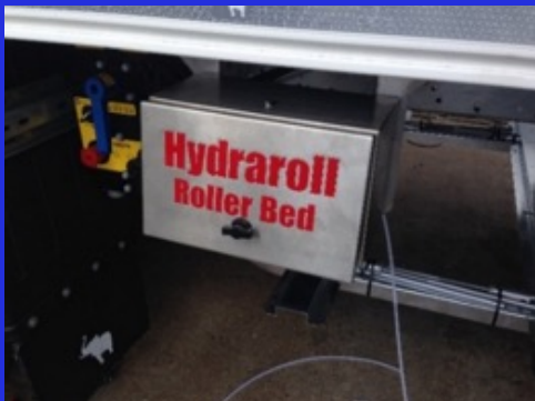
STAINLESS STEEL CONTROL BOX UNDERNEATH VEHICLE
